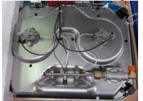
7. Clean bottom of main top near regulator with a 50/50 mixture of rubbing alcohol and water.
